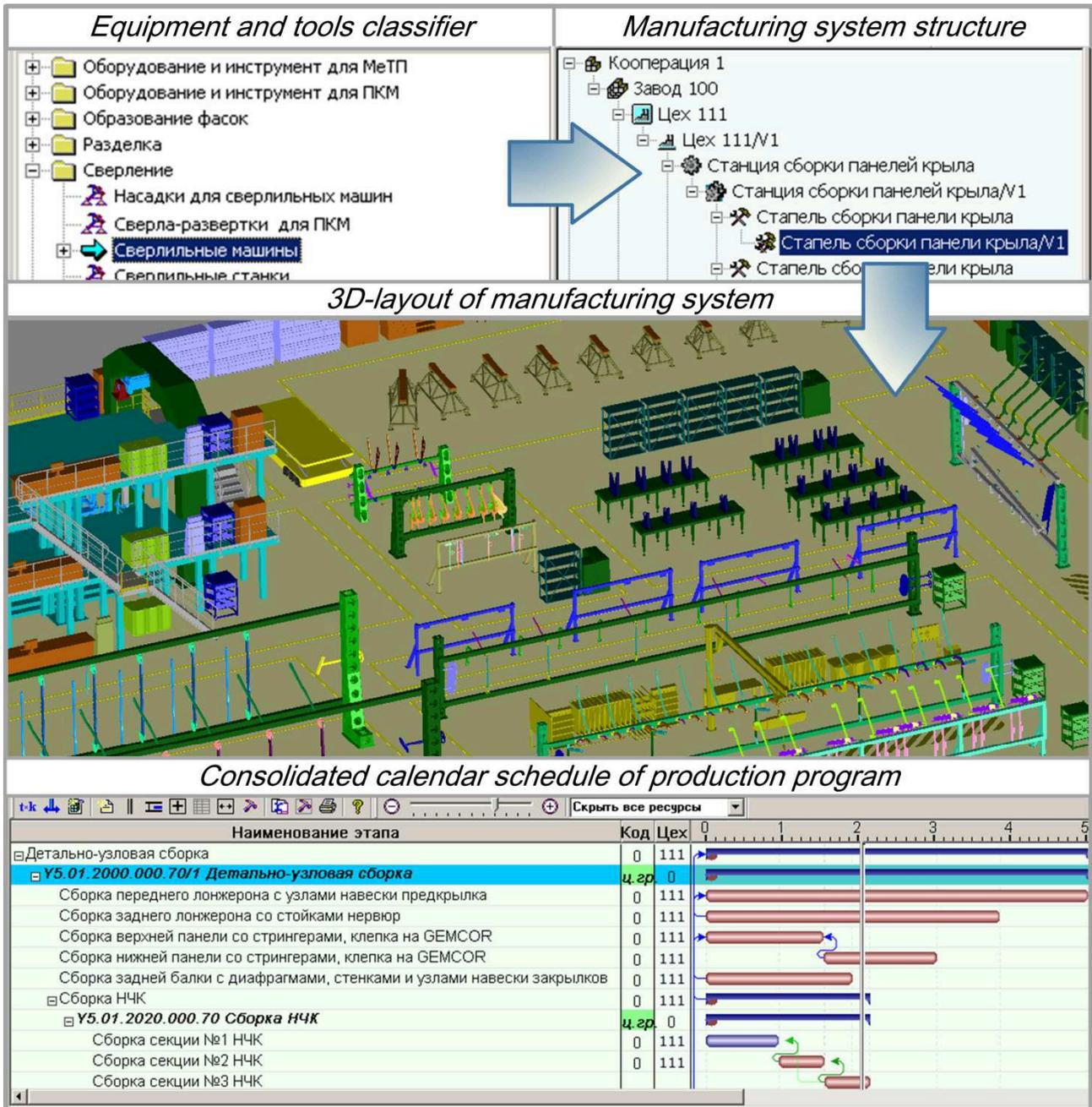
Fig.3. Assembly production simulation model.
