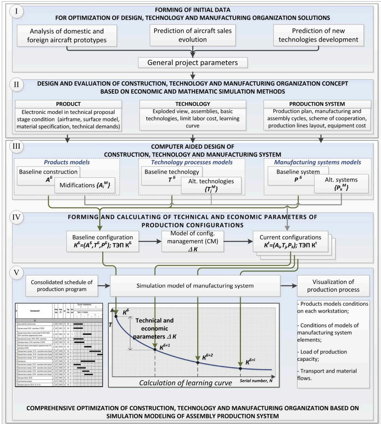
Fig.1. Scheme of making and optimization of construction, technology and manufacturing organization decisions of assembly production.
